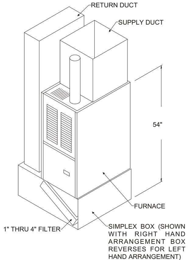
**Caution: SOME FURNACES DO NOT COVER OPENING COMPLETELY ON SIMPLEX BOX. A FIELD SUPPLIED SHEET METAL BLOCK OFF PLATE MUST BE USED TO SEAL THE OPENING.**
